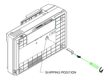
Figure 2-1 Removing the Shipping Bracket
